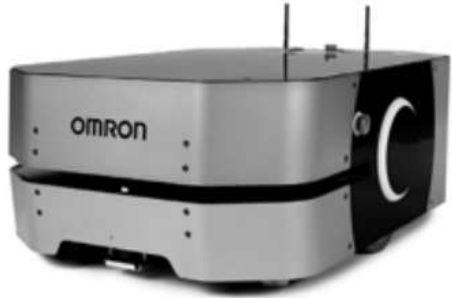
Autonomous Mobile Robot logistics system (AMR)
