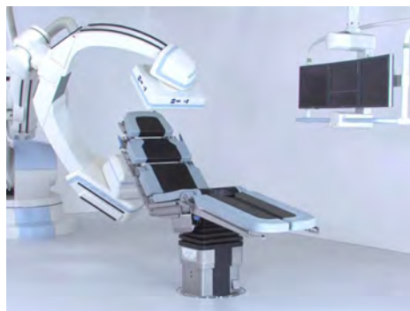
Fig. 14. Integrated Trumpf OR table with breakable tabletop and metal parts that impair image quality
