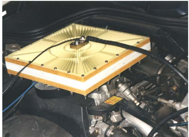
Fig. 1: Starting a Mercedes C220 with a 30 V/65 F supercapacitor (bipolar metal oxide technology, 4 Wh/l, 1.3 Wh/kg).
