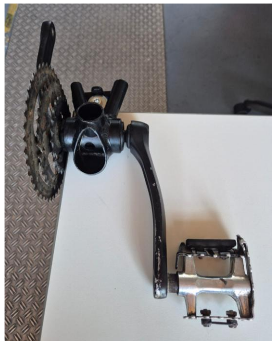
Figure 20: Prepared bicycle crank for the drive (Own photograph)
