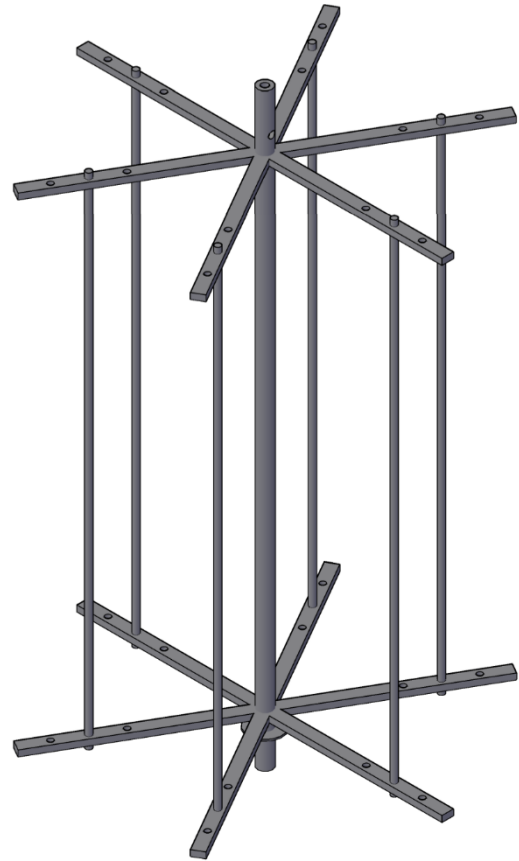
Figure 16: 3D CAD model of the hose holder (Own CAD model)
