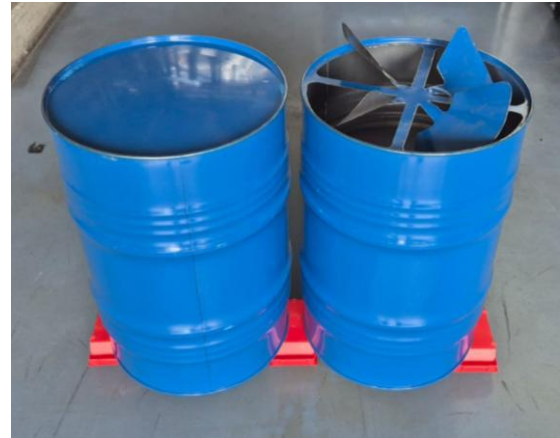
Figure 64: Bottom view of metal barrels before processing (left) and after manufacturing of the turbine blades (right) (Own photograph)
