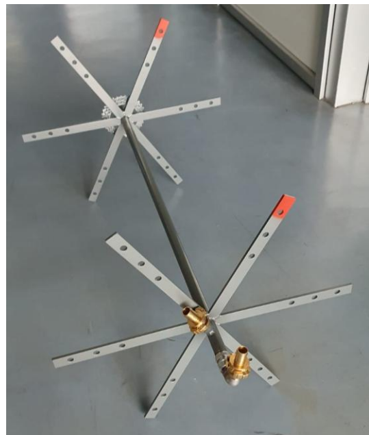
Figure 18: Hose holder after coating and colouring (Own photograph)
