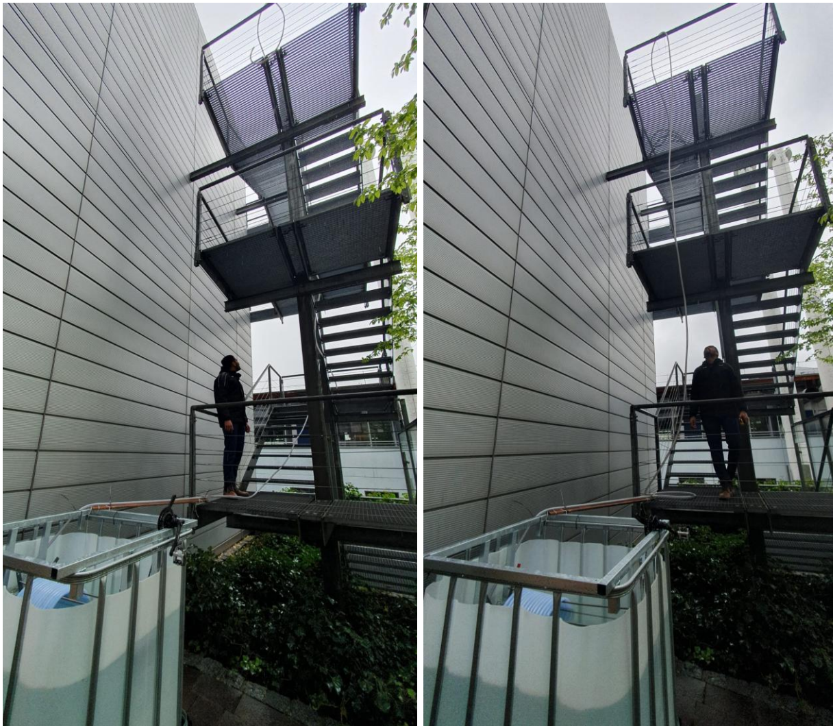
Figure 25: Horizontal configuration of the stationary hose as variant 1 via the stairs (left) and as variant 2 straight up (right) (Own photographs)
