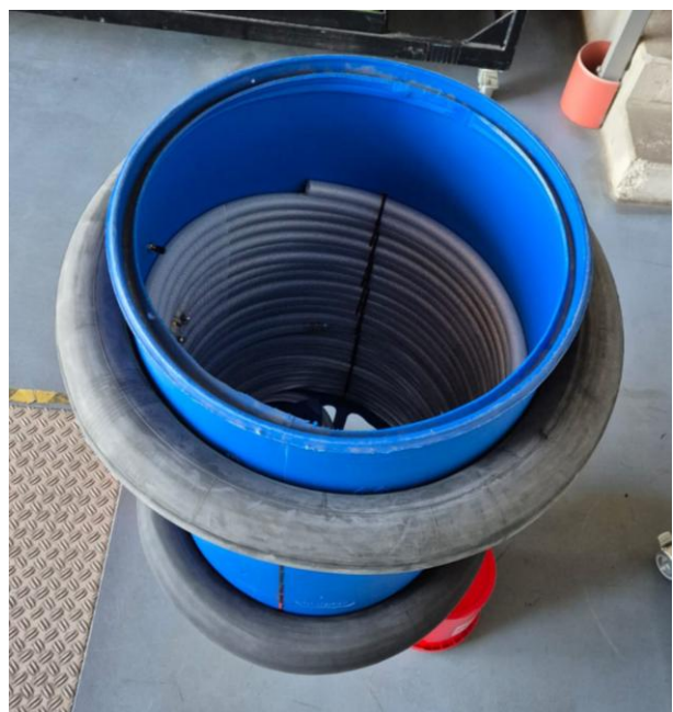
Figure 72: Pump with the motorcycle inner tubes attached from behind (Own photograph)
