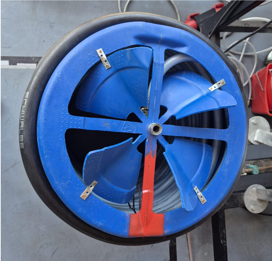
Figure 69: First version of the pump prepared for testing (front view) (Own photograph)
