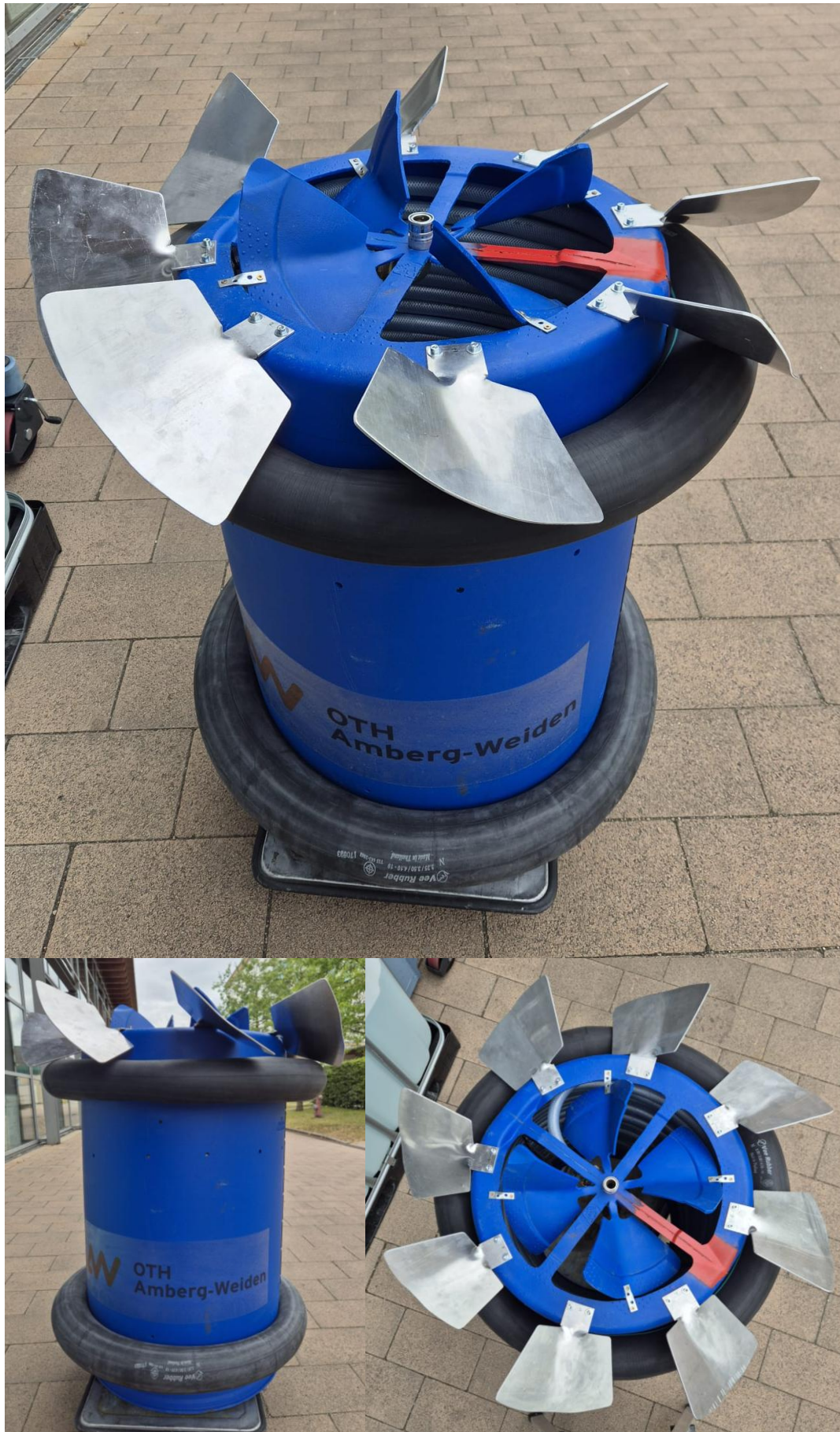
Figure 74: Optimised version of the pump prepared for testing from different angles (Own photographs)
