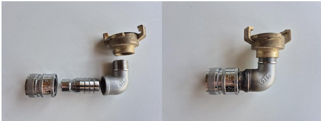
Figure 17: Transition from the shaft to the stationary hose as individual parts (left) and assembled (right) (Own photograph)
