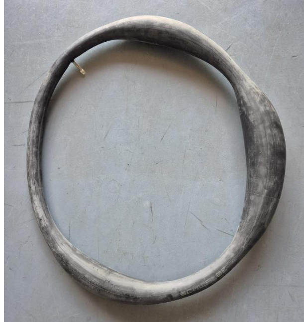
Figure 67: Uneven shape of an inflated bicycle tube (Own photograph)
